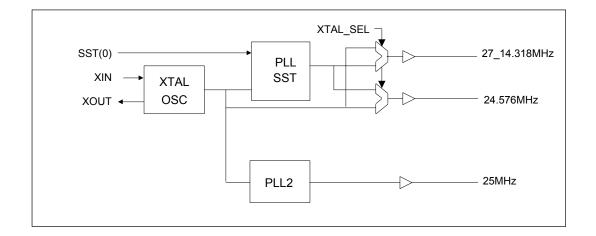
Note: Only 27MHz output is modulated for low EMI via Spread Spectrum.
